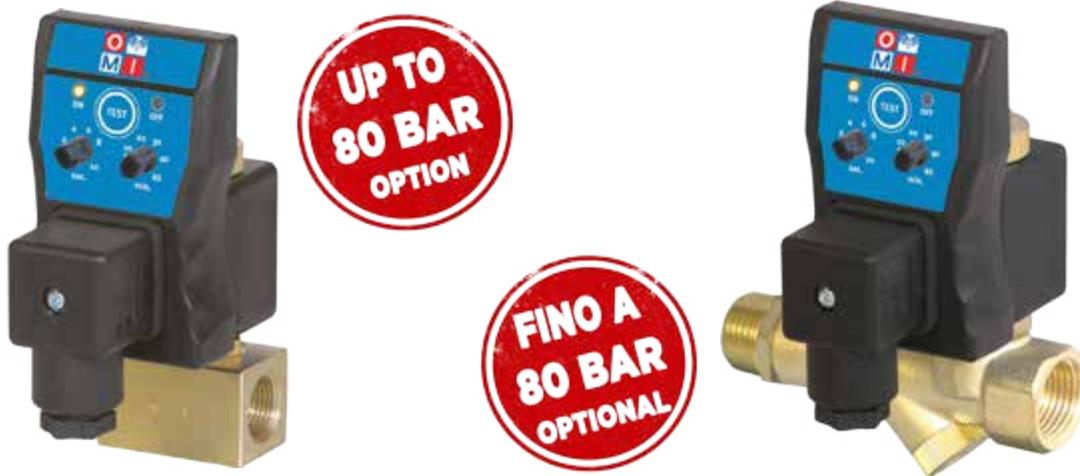
The SC-TIMED timer controlled condensate drain is a combination of a solenoid valve and an electronic timer designed to automatically remove condensate from compressed air systems. The SC-TIMED COMBO in addition, has an integral ball valve and a strainer, all in the same body.
