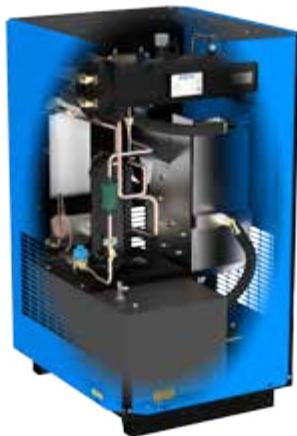
The refrigeration circuit cools the glycol in the tank and this thermal mass cools compressed air inside the heat exchanger.
