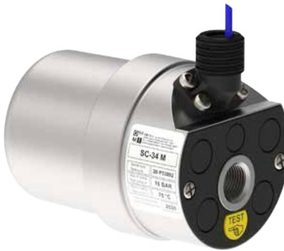
The SC-12 and SC-34 float drains models combine ease of use, functionality and robustness. They are also extremely versatile, as they are suitable for working with compressor capacities up to 8000 m<sup>3</sup>/h, do not require electricity and can be installed to discharge the condensate from compressed air vessels, filters, condensate separators and dryers.
