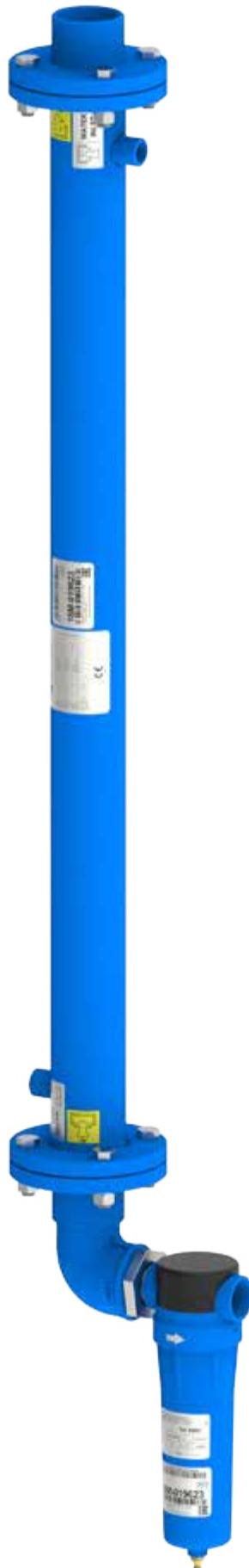
The water after-coolers are composed of two parts: a high efficiency shell in tube air-water heat exchanger, offering little pressure drops to cool air, and a cyclone condenser separator to separate and eliminate the condensed water.
